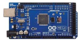
Figure 3.1. Arduino Mega
